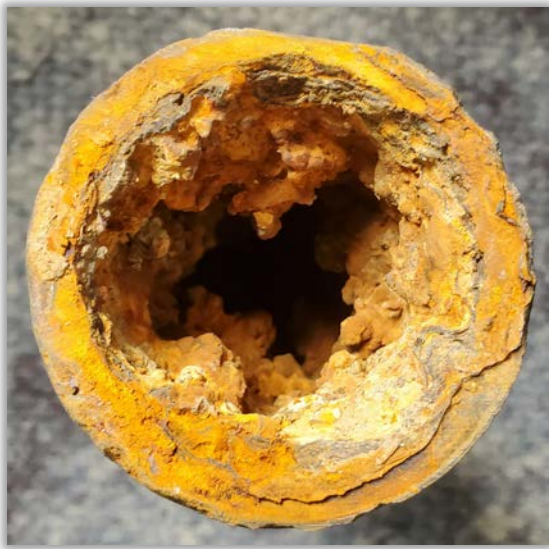
Corroded & Aging Smithville Waterline Segments
